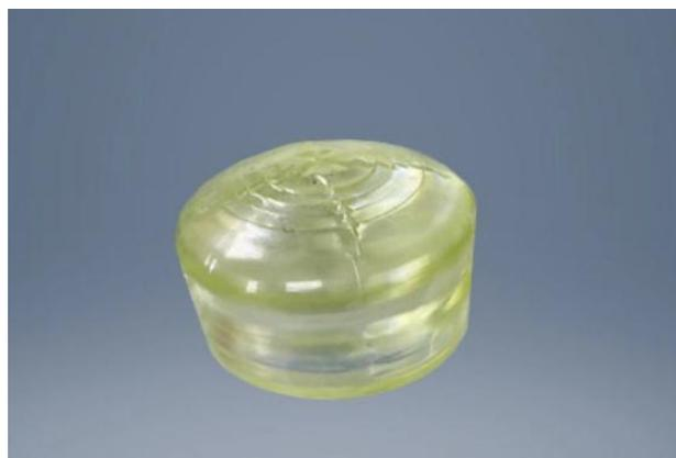
Lithium Niobate is an inorganic material, chemical formula LiNbO<sub>3</sub>, is a negative crystal, ferro-electric crystal, polarization of lithium niobate crystal with piezoelectric, ferro-electric, photoelectric, nonlinear optical, thermo-electric materials, and have optical refractive effect.
